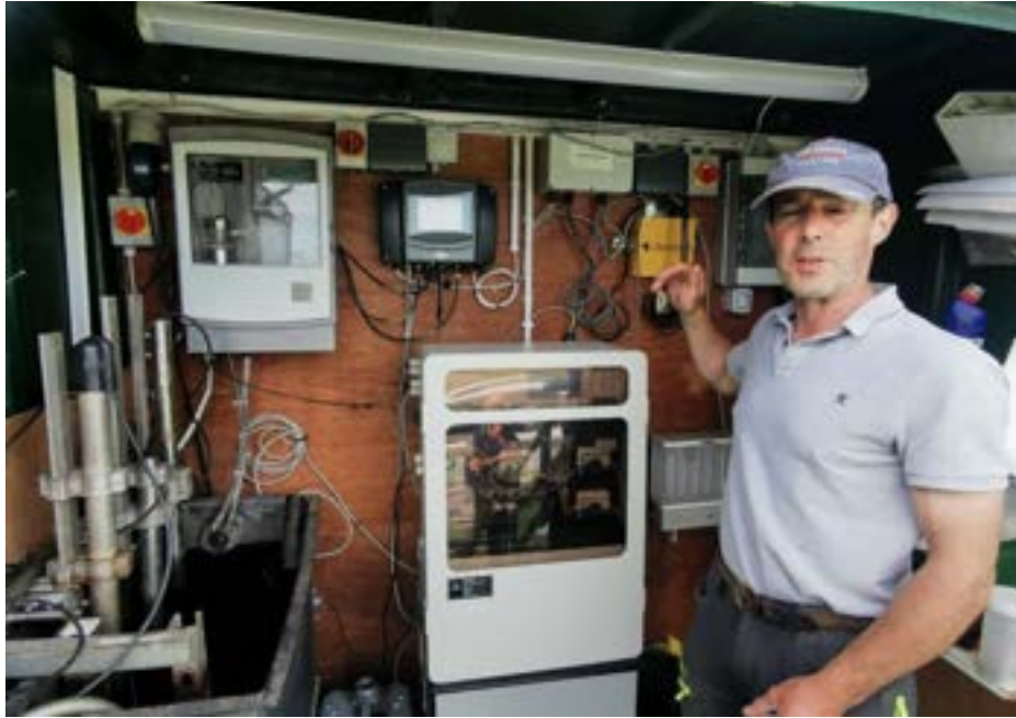
Real time water sensing, including nitrate and phosphate, on streams in Ireland
